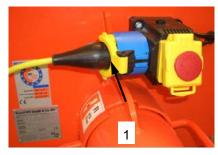
Fig. 25: Electrical connection
