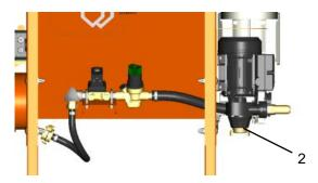
Fig. 15: Water connection with a booster pump
