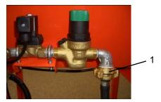
Fig. 14: Water connection without a booster pump
