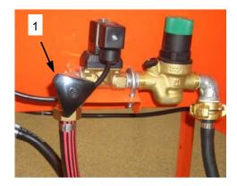
Fig. 30: Water outlet valve
