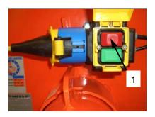
1. Switch off the machine at the red "OFF pressure switch.
