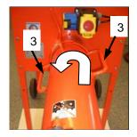
Fig. 37: Removing the mixing tube
